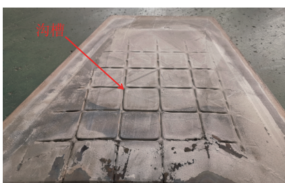
图4 蒙皮表面形成的沟槽 Fig.4 Grooves formed on surface of the panel
